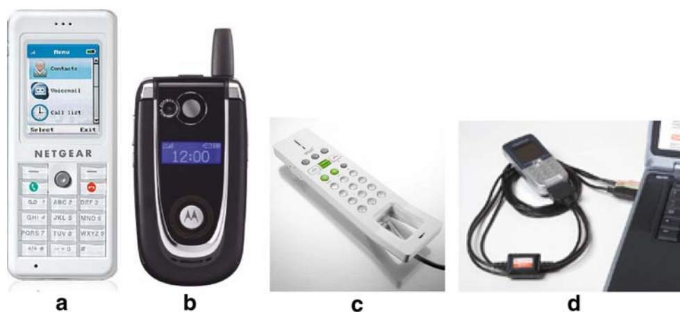
Fig. 3 Skype gadgets: (a) Netgear Skype Wi-Fi phone, (b) Motorola CN620 Skype Wi-Fi phone, (c) IPEVO Free-1 USB Skype phone, and (d) IPdrum mobile Skype cable
